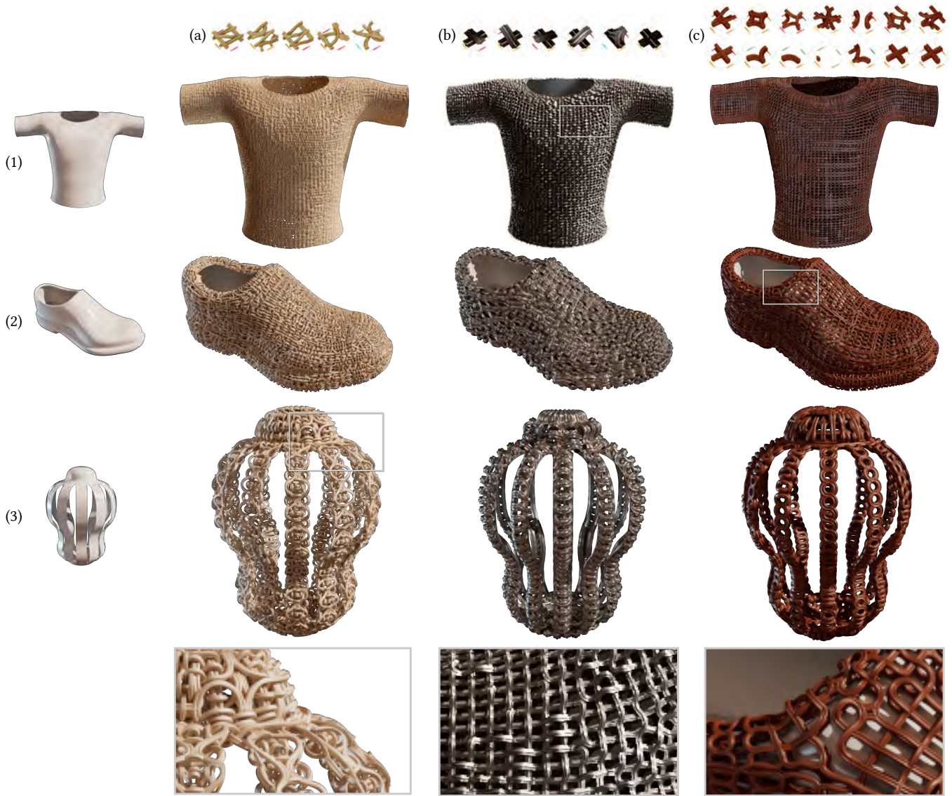
Figure 9: Once designed, the same tile set can be applied to various macrosurfaces.
