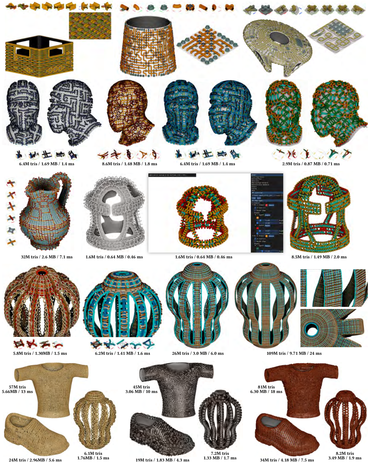
Figure 11: Additional results illustrating the variety of mesostructures achievable with our system, captured from our real-time generated mesostructures. For each example, we report the amount of synthesized polygons, the GPU memory footprint of our procedural model and the render time on an Nvidia RTX 3070 Ti device for 720p images. The last row corresponds to the beauty shots of Fig. 9 and the examples of Tab. 1.
